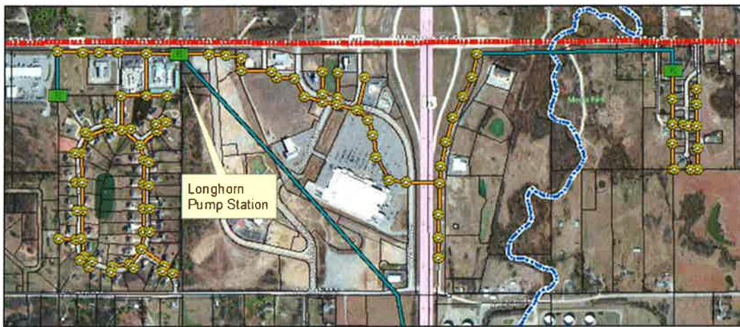
Figure 3-1: Longhorn Lift Station Contributing Collection System
