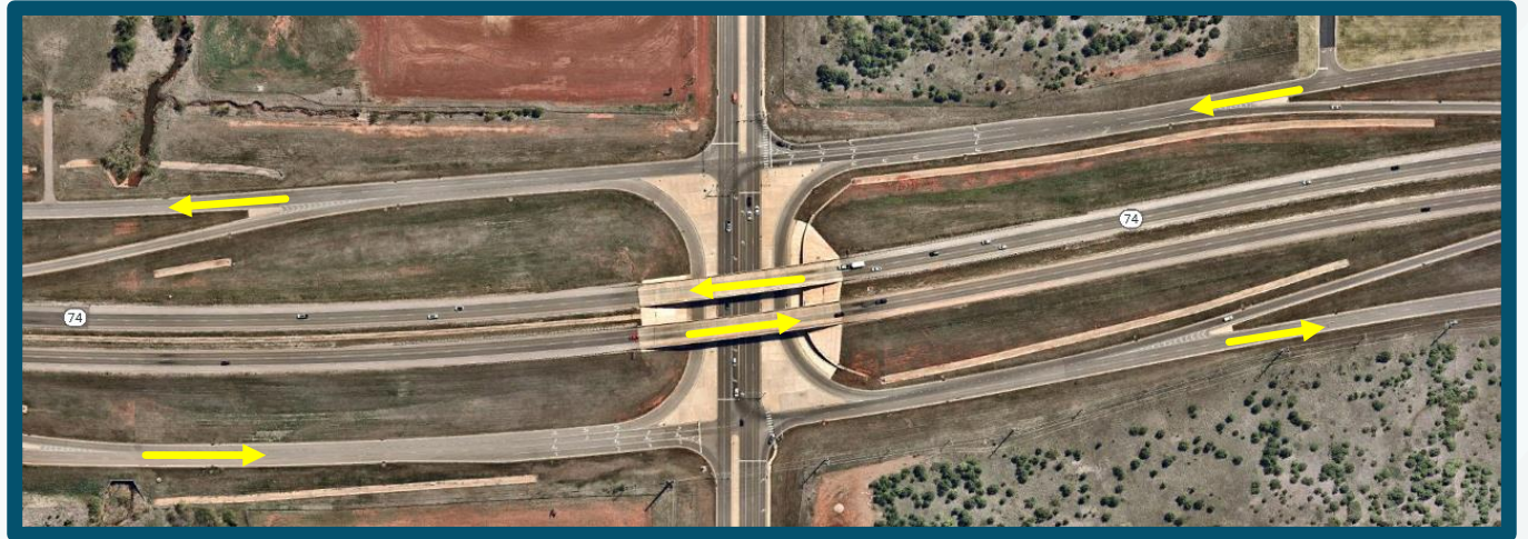
Grade Separated Highway with Frontage Road Example
