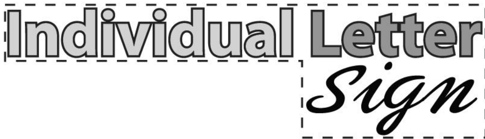
Figure 60-3: Sign Area Measurement (Individual Letter Signs)
